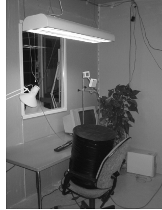
Figure B.5 The test room in the laboratory measurements. The room was constructed to simulate the conditions of a common cell office room. A placement of heat loads: computer, dummy and lighting can be seen on the right photo.
