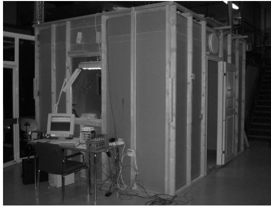
Figure B.5 The test room in the laboratory measurements. The room was constructed to simulate the conditions of a common cell office room. A placement of heat loads: computer, dummy and lighting can be seen on the right photo.
